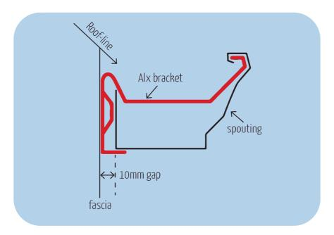
In 2011 and in response to NZ's leaky home problem, the NZ Standards Authority rewrote their guidelines for spouting. In this, they called for an overflow provision to minimise the chance of water flowing back into a building.
